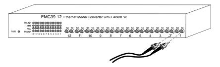
Figure 3-2 Connecting a Fiber Link to the EMC39-12
